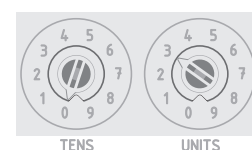
Figure 10: Decade address switches address 03 selected
